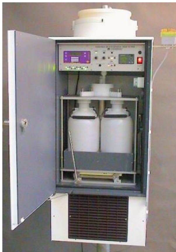
NSA 181/KD - VMM Including data logging system
