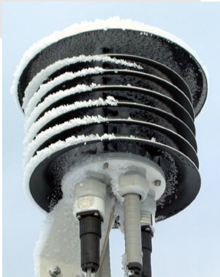
Lamellar Shelter LAM 630 with temperature and humidity sensors
